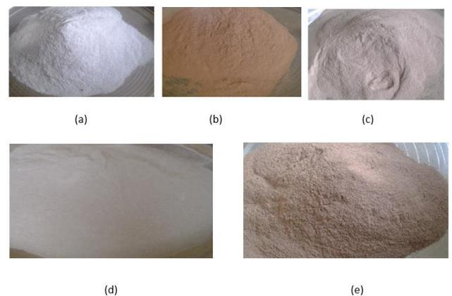
Fig. 1. Ground Construction Waste Materials (a) Waste glass Powder (b) Waste Brick Block Powder (c) Waste Brick Tile Powder (d) Waste Sandcrete Hollow Block Powder (e) Synergy of (a), (b), (c), and (d)
