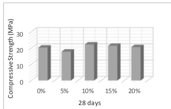
Fig. 5. Compressive Strengths of concrete at 28 days
