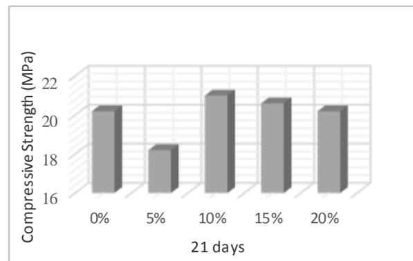
Fig. 4. Compressive Strengths of concrete at 21 days
