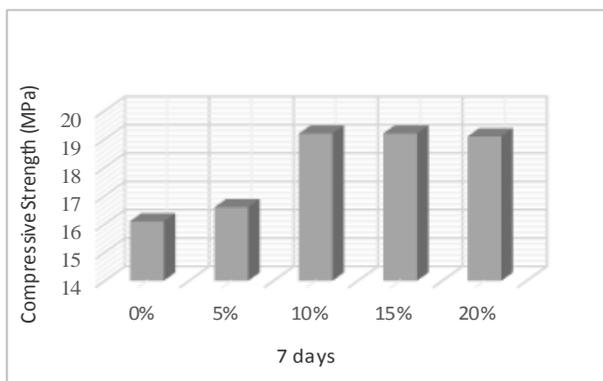
Fig. 2. Compressive Strengths of concrete at 7 days
