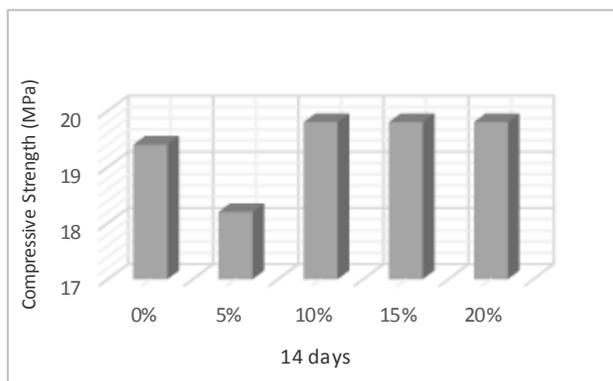
Fig. 3. Compressive Strengths of concrete at 14 days
