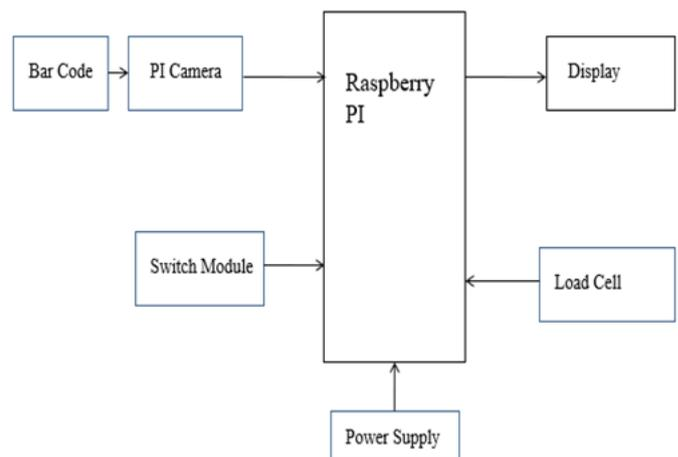
Fig. 1. Block Diagram of Smart Shopping Trolley
