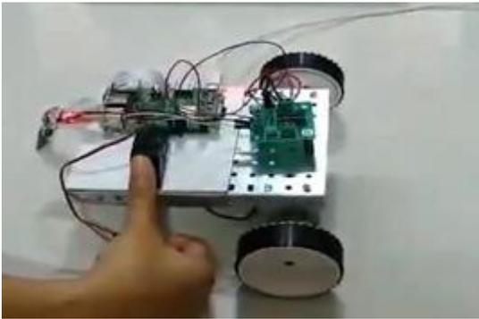
Fig. 6. Providing input to the system through fingerprint scanner.
