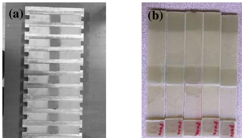
Figure 2. Preparation of Adhesive Single Lap Joints; a) Sticking the Composite Substrates, b) Test Samples
