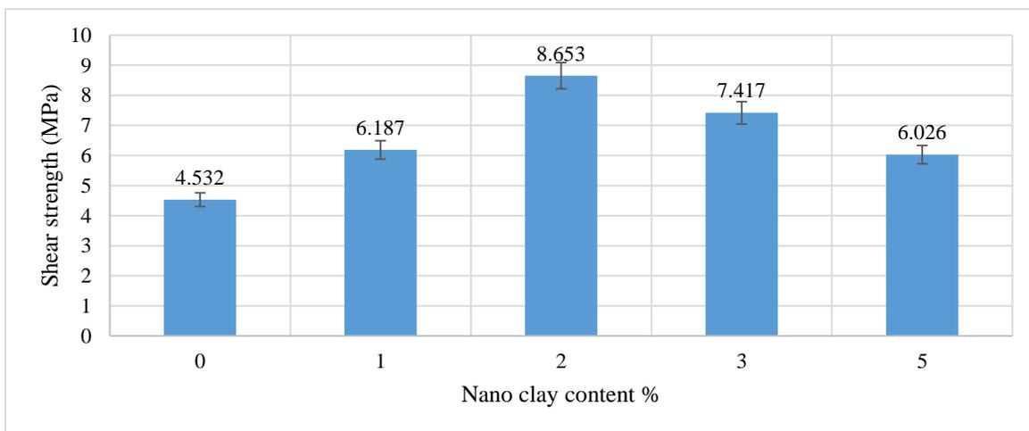
Figure 6. Maximum Shear Strength of SLJs versus CNP Weight Content
