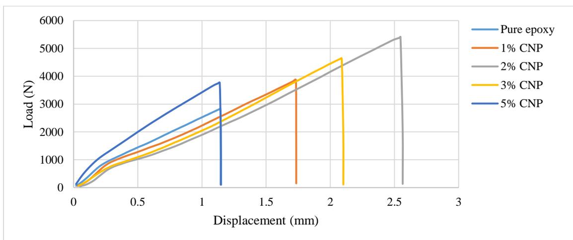
Figure 4. Load-Displacement Curves for SLJs Reinforced with Different Amount of CNP and Subjected to Tensile Loading
