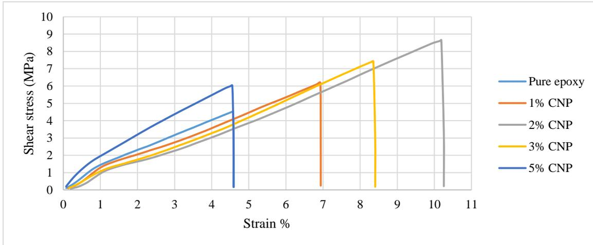
Figure 5. Shear Stress-Shear Strain Curves for SLJs Reinforced with Different Amount of CNP and Subjected to Tensile Loading
