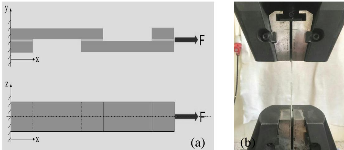
Figure 3. Illustration of Lap Shear Test; a) Boundary Conditions, b) Tensile Loading
