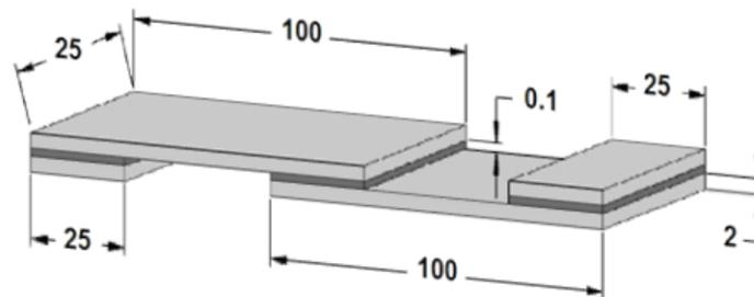
Figure 1. Single Lap Joint Configuration with Dimensions in (mm)
