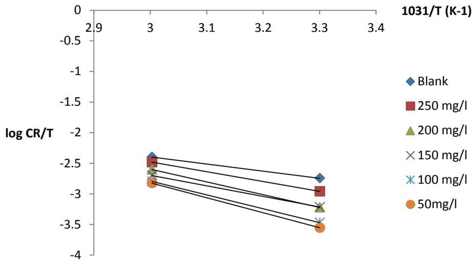
Figure 3: Arrhenius plots for the mild steel dissolution in the absence and presence of *Cajanus cajan* leaves extract
