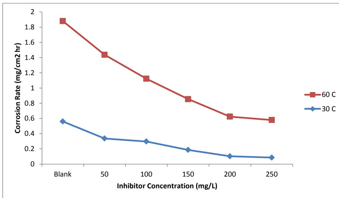
Figure 1: Corrosion Rate of Mild Steel in 3.5 wt.% NaCl solution in the absence and presence of *cajanus cajan* leaves extract at various temperatures
