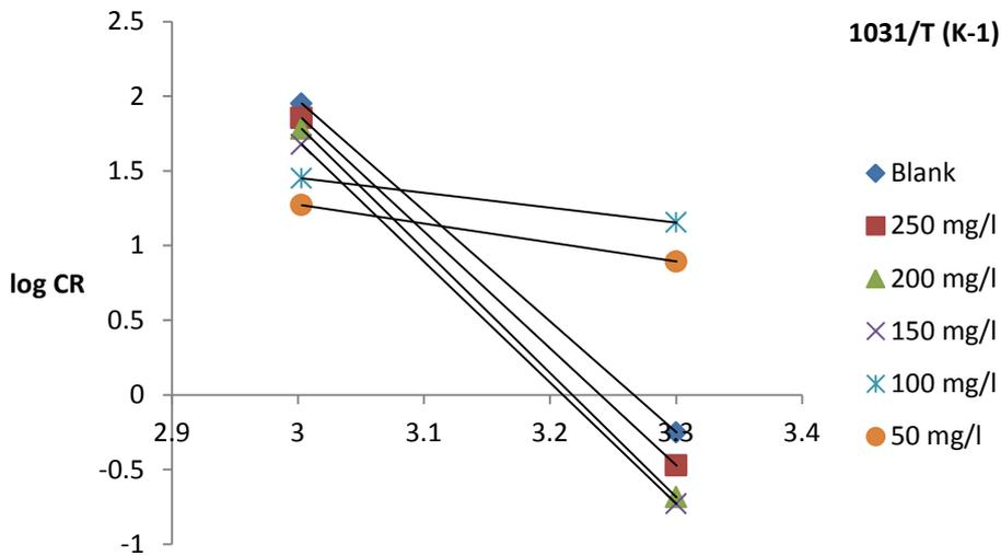
Figure 4: Activation energy plots for the mild steel dissolution in the absence and presence of *Cajanus cajan* leaves extract
