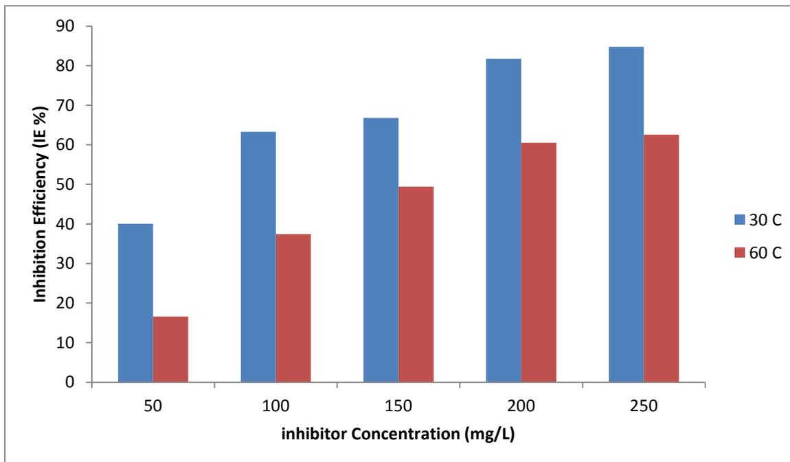
Figure 2: Inhibition Efficiency of Mild Steel in 3.5 wt.% NaCl solution in the absence and presence of *cajanus cajan* leaves extract at various temperatures
