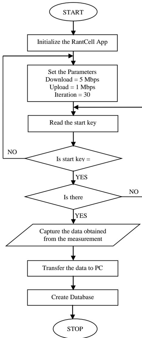
Figure 2: Data Acquisition Flowchart
