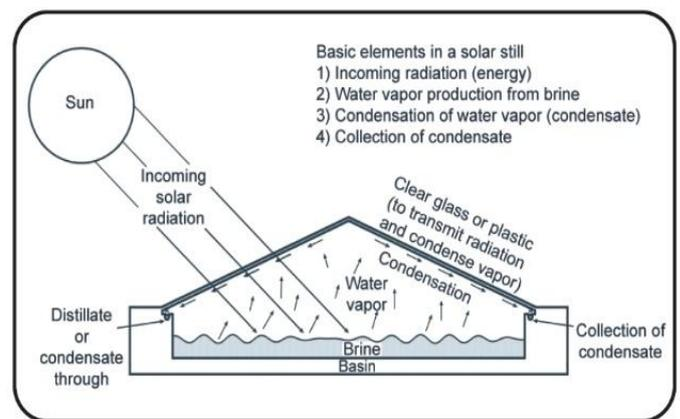
Fig. 1. Conventional Solar Desalination
