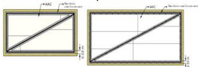
Fig. 4. AAC wall panel specimens with bamboo reinforcement
