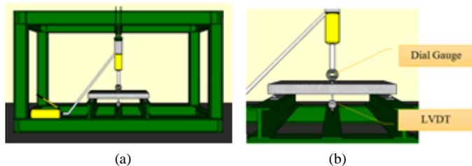
Fig. 5. (a) Tool setting and testing specimen (b) the close detail
