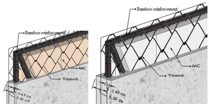
Fig. 3. AAC wall panel specimens with bamboo reinforcement
