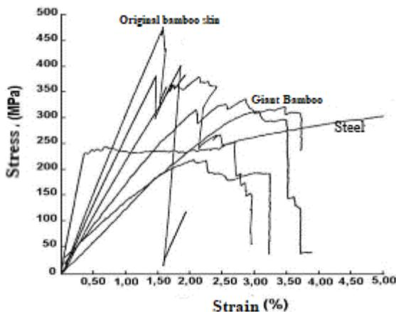
Fig. 1. Test Results of Bamboo and Steel Tensile Strength Baja (Morisco, 1999)
