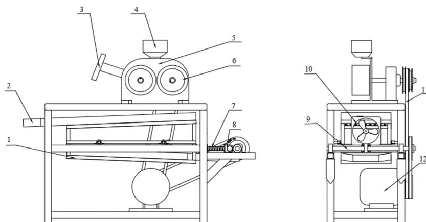
Figure 5: Structure of a salvia seed coat separator
