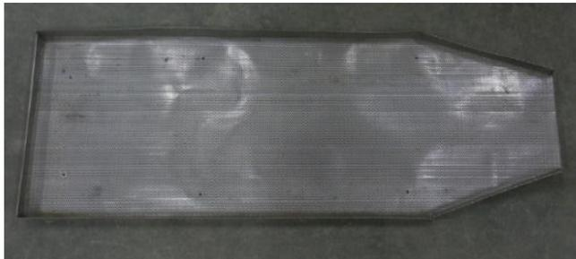
Figure 6: Vibrating screen after manufacture.
