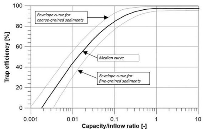
Fig. 3. Efficiency Trap Curve.
