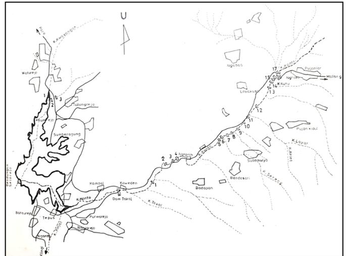
Fig. 11. Sabo dam layout and check dam upstream of the Selorejo reservoir
