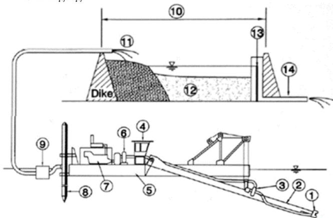
Fig. 4. Schematic diagram of a hydraulic dredger and disposal area.
