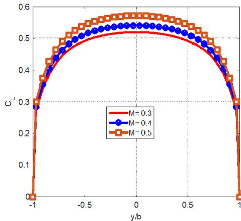
Figure 4. Lift coefficient on wingspan  $M_\infty = 0.3; 0.4; 0.5$ .
