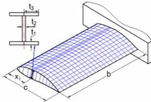
Figure 3. Structure of the wing with ribs and rib spars
