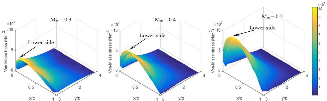
Figure 6. Stresses at the upper side and lower side of wings when  $M_\infty = 0.3; 0.4; 0.5$ .
