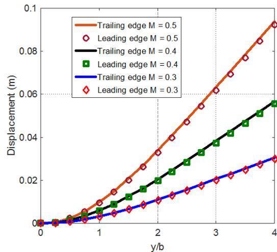
Figure 5. Displacement at the leading and trailing edge  $M_\infty = 0.3; 0.4; 0.5$ .
