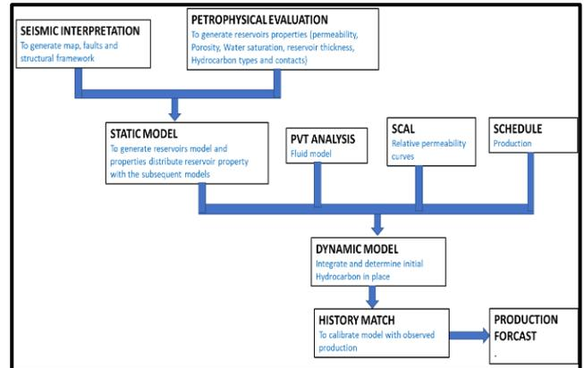
Fig. 1. Simulation Flow Chart
