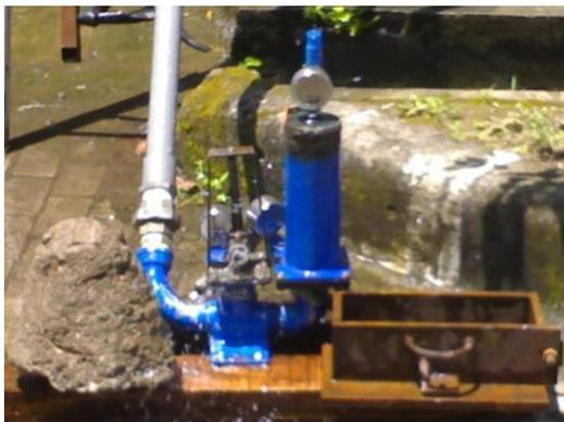
Fig. 1. Hydam pump with ILK pump arrangement
