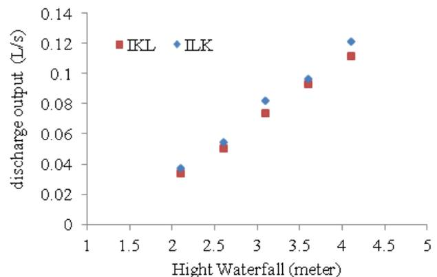
Fig. 4. Graph of the relationship between the height variations that occur in the discharge of output in the ILK and IKL arrangement
