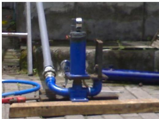
Fig. 2. Hydam pump with IKL pump arrangement
