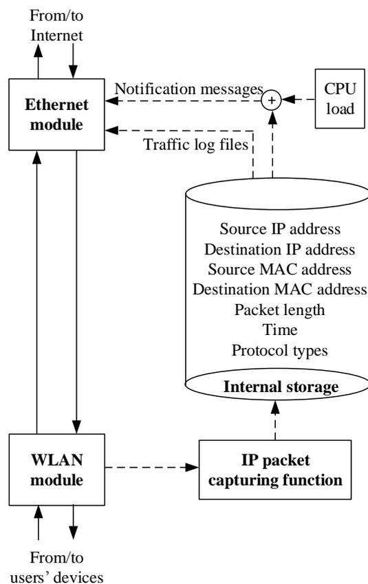
Fig. 2. Conceptual illustration of the proposed access point’s function.
