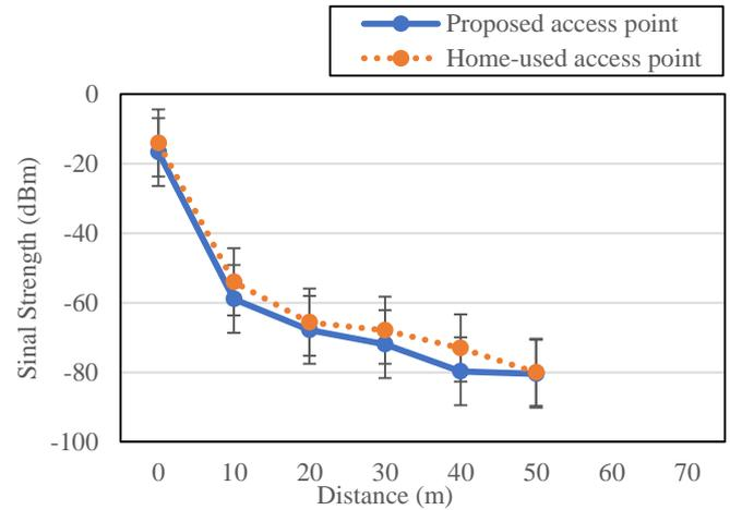
Figure 8: Signal Strength versus distance between access points and user device.
