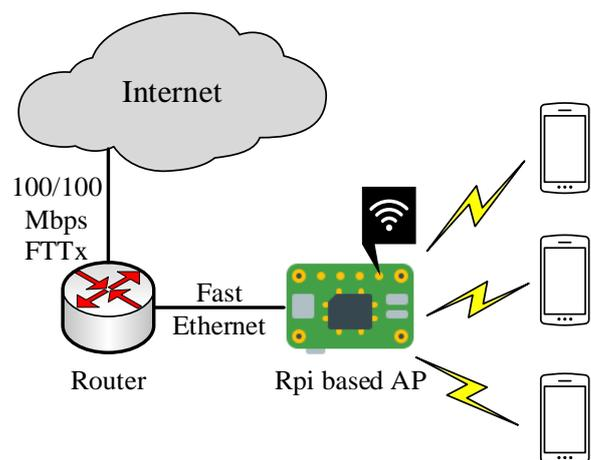
Fig. 3. Network configuration environment.
