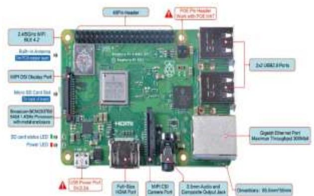
Fig. 1. Components of Raspberry Pi 3 B+ [4].
