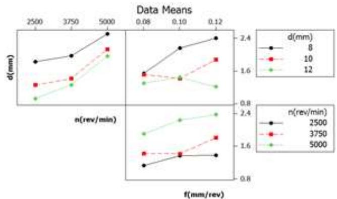
Fig. 5. Interaction plot for R<sub>a</sub>
