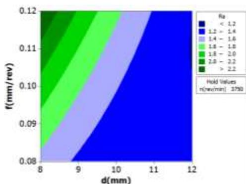
Fig. 8. Contour plot of  $R_a$  vs  $f$  (mm/rev),  $d$ (mm)
