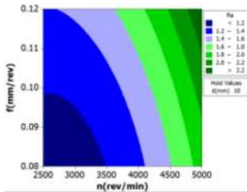
Fig. 7. Contour plot of  $R_a$  vs  $f$  (mm/rev),  $n$ (rev/min)
