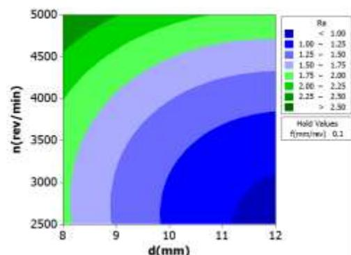
Fig. 6. Contour plot of R<sub>a</sub> vs n(rev/min), d(mm)
