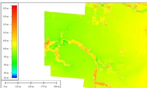
Fig. 5. The Bare Earth by Slope 5°, Radius 1m Method.
