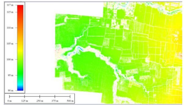
Fig. 7. The Bare Earth by Slope 0.50 radius 10m method
