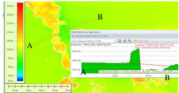
Fig. 6. Profile elevation a Segment A to B
