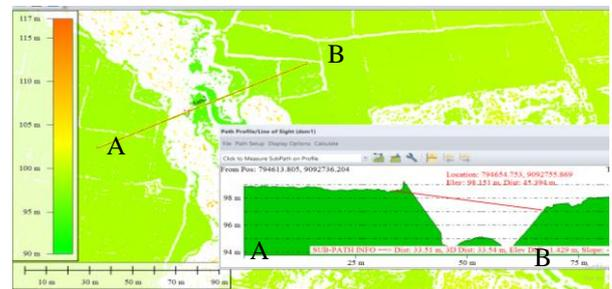
Fig. 8. Profile bare earth by slope 0,50 and radius 10m A to B
