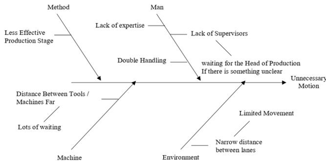
Fig. 7. Unnecessary motion.
