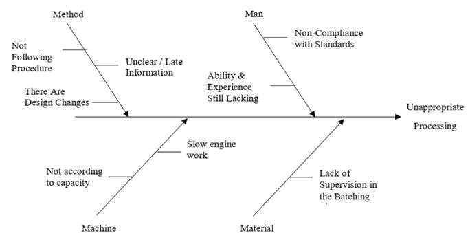
Fig. 6. Unappropriate processing.
