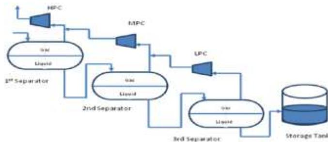
Figure 2. Simplified schematic of the optimized X-Field's surface production facility [3].
