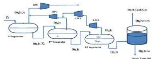
Figure 1. Simplified schematic of the modeled X Field's surface production facility [3].
