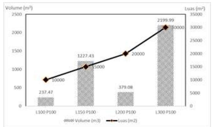
Figure 10. Graph of Relationship between Sediment Volume and Sediment Area Detained in Each Scenario (3 Months)
