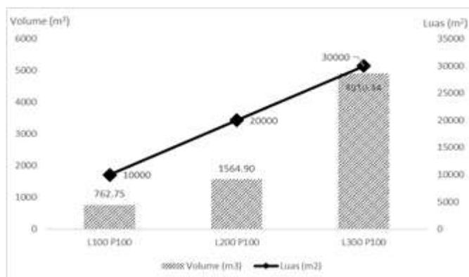
Figure 9. Graph of Relationship between Sediment Volume and Sediment Area Detained in Each Scenario (1 Month)
