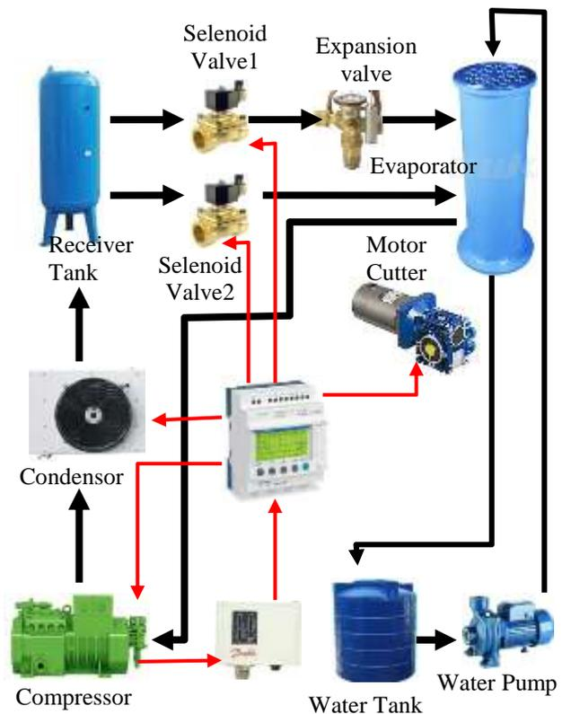
Figure 1. Work diagram of a crystal ice machine
