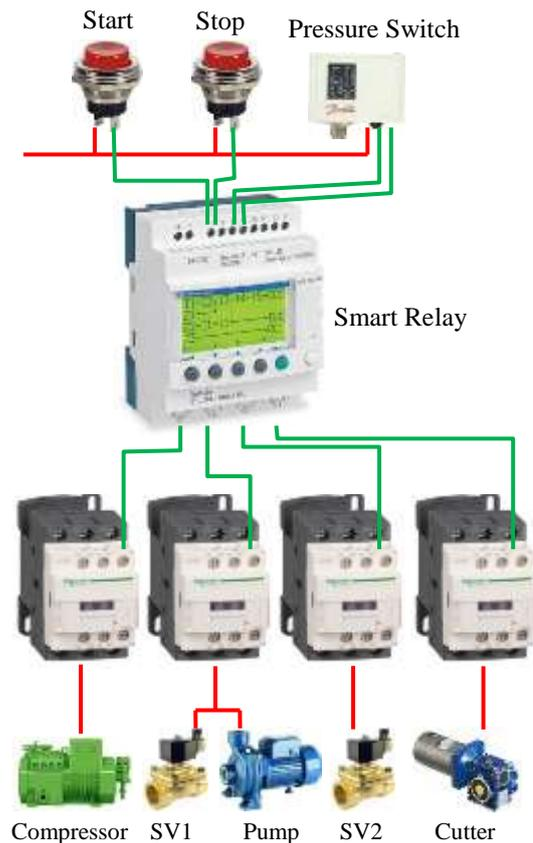
Figure 4. Single Line Diagram
