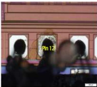
Fig. 1. Bond pad contamination
