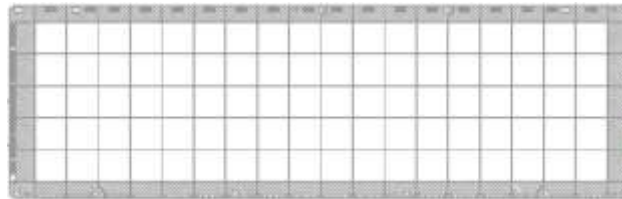
Fig. 1. Single panel large substrate strip for MEMS package.
