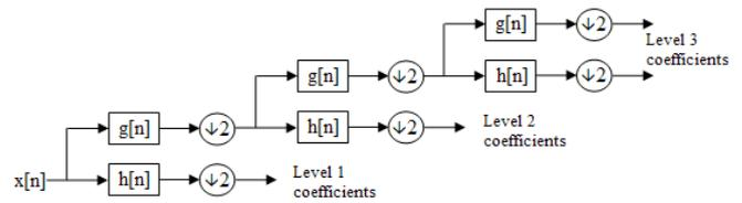
Fig. 2. A three-level wavelet filtering
