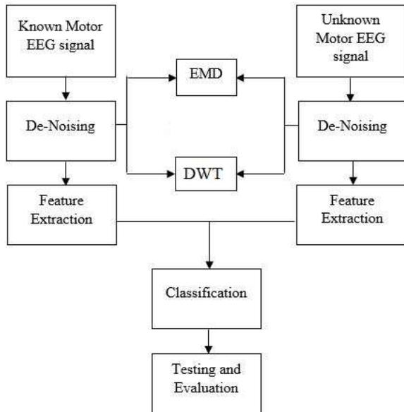
Fig. 1. Proposed Model work flow diagram
