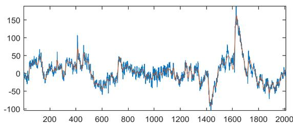
Fig. 4. De-noised signal using EMD (Blue=Original Signal, Orange=De-noised Signal)
