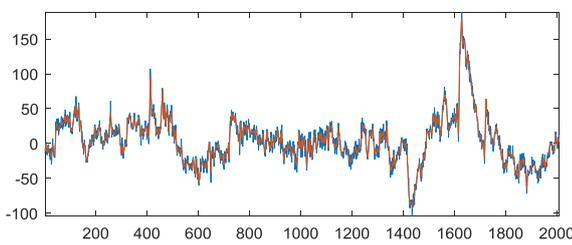
Fig. 5. De-noised signal using DWT (Blue=Original Signal, Orange=De-noised Signal)
