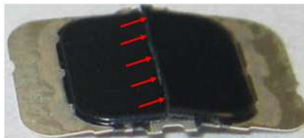
Fig. 2. Package crack due to package bending of a very thin package.
