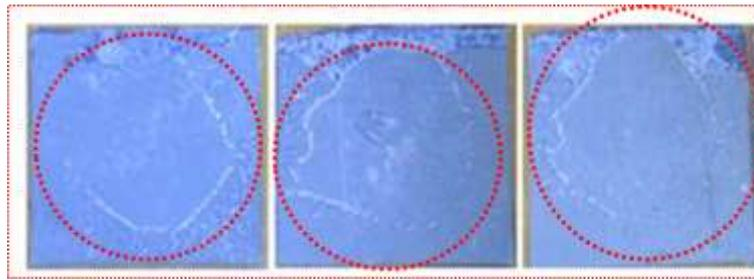
Fig. 6. Optical Photo of DAF Voids
