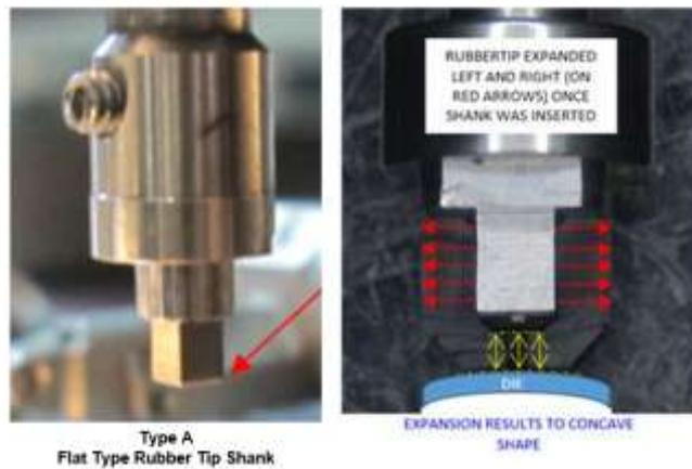
Fig. 3. Flat Type Rubber Tip Shank
