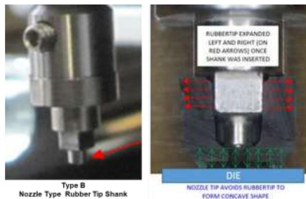
Fig. 7. Nozzle Type Rubber Tip Shank
