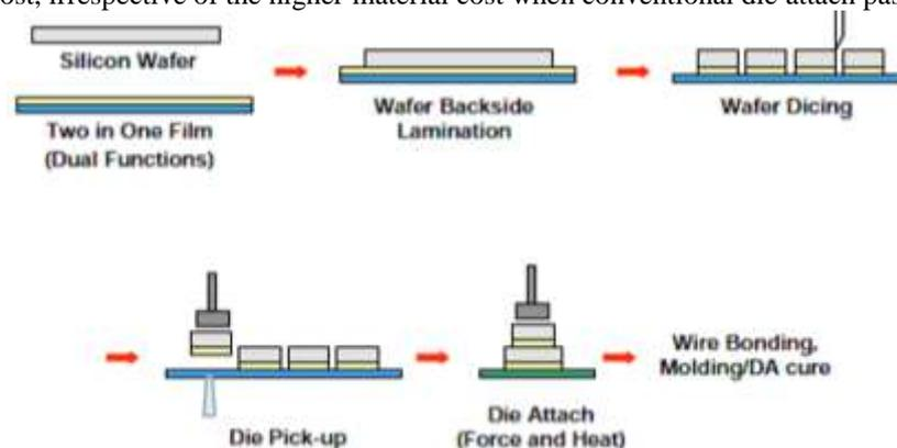
Fig. 2. Dicing Die Attach Film Assembly Process
