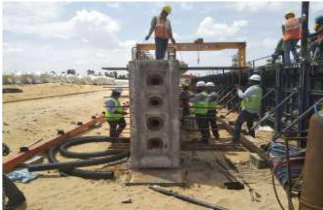
Fig. 3. View of the Upv Test In Progress In A Psc Girder By Direct Method Of Measurement
