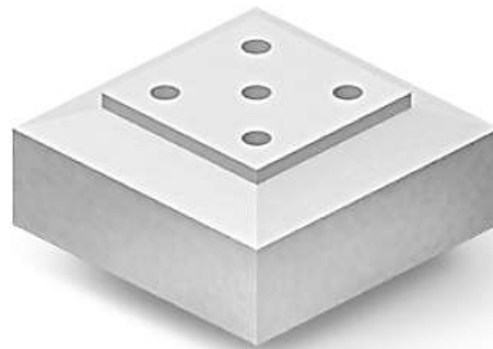
Fig. 7. DA Pick-up tool with distributed vacuum hole design
