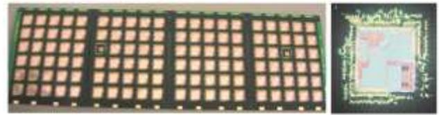
Fig. 2. LFBGA273 wire bonded sample
