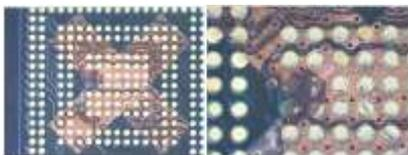
Fig. 14. Mold compound bleeding the backside from supplier reject
