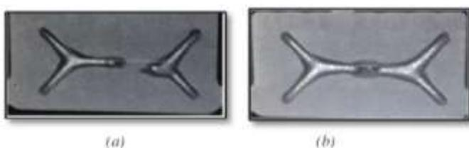
Fig. 9. Epoxy pattern formation at (a) 3.7 mm/s and (b) 3.9 mm/s
