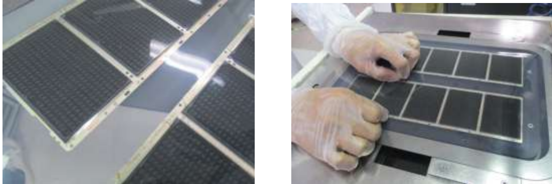
Fig. 3.0 Operator applied pressure on area of strip package affected by weak adhesion.
