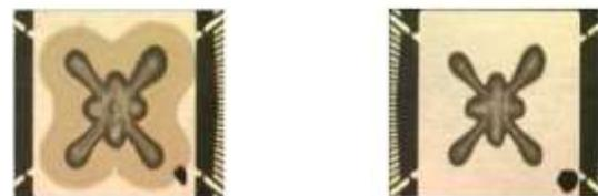
Figure 4. Result of Plasma Cleaning
