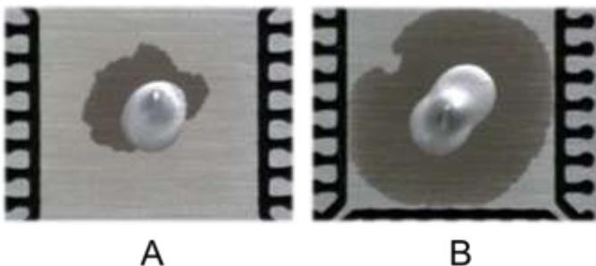
Figure 1. Example of Resin bleed-out (RBO)
