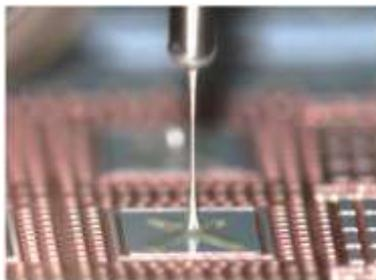
Fig. 2. Excessive Epoxy tailing and Epoxy on Leads failure mechanism
