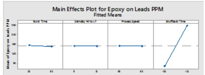
Fig. 8. Main Effect plot for Epoxy on leads
