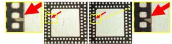
Fig. 4. Epoxy on Leads at Visual Inspection
