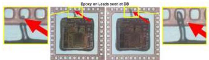
Fig. 3. Epoxy on Leads at Die Bond
