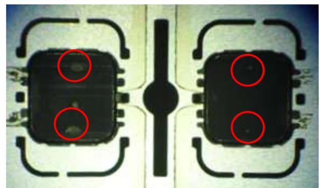
Figure 8. Package voids defect signature
