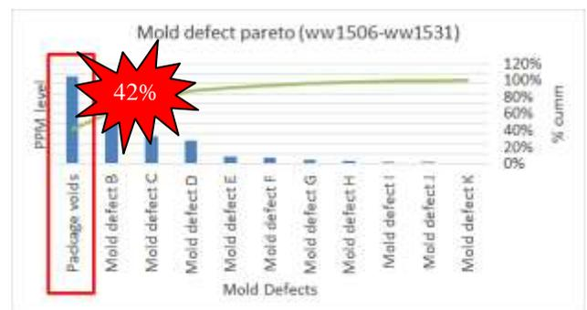
Figure 3. Mold defect pareto
