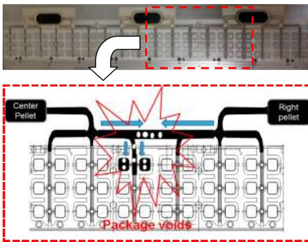
Figure 15. Package voids defect mechanism
