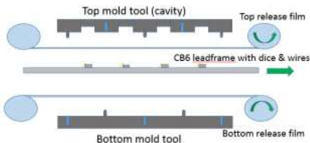
Figure 4. Reel-to-reel film-assisted transfer molding configuration
