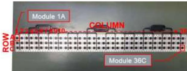
Figure 9. Module location identification
