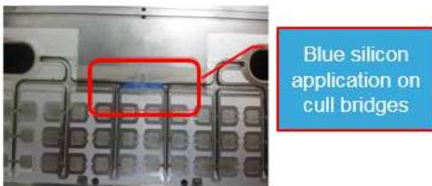
Figure 16. Temporary blocking of cull bridges
