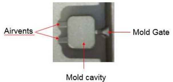
Figure 6. Individual module cavity
