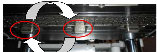
Figure 14. Center plunger swapped with Left plunger
