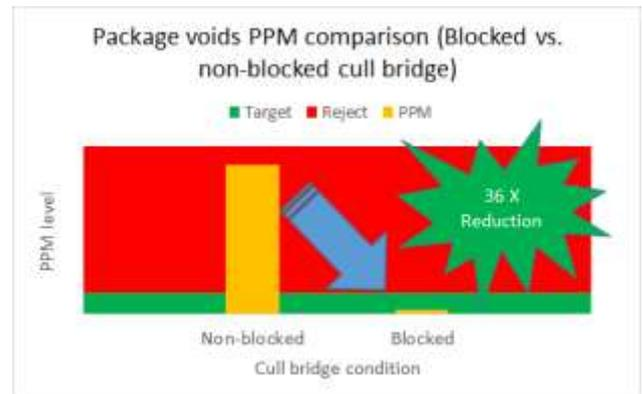
Figure 17. Blocked vs non-blocked cull bridge validation summary
