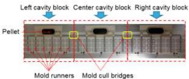
Figure 5. Top mold tool configuration
