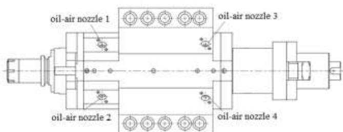
Fig. 4. Front projection of main spindle illustrates the schematic position of oil-air nozzles.
