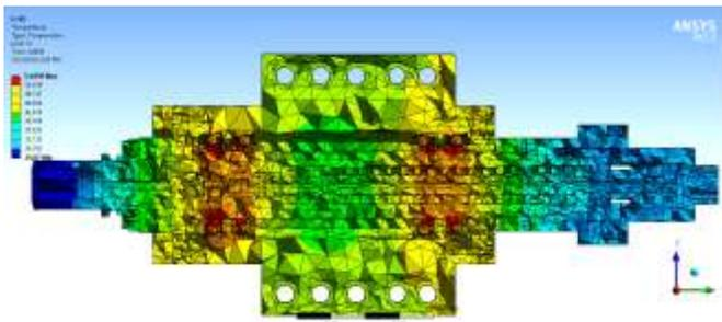
b. Thermal distribution in the spindle components at the cross section through the center axis of the spindle.
