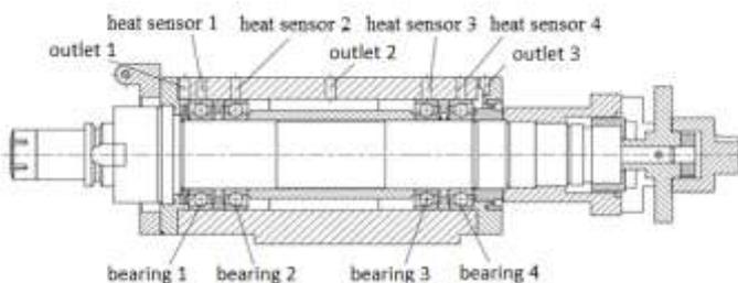
Fig. 3. Schematic illustration of air outlet and temperature sensor.
