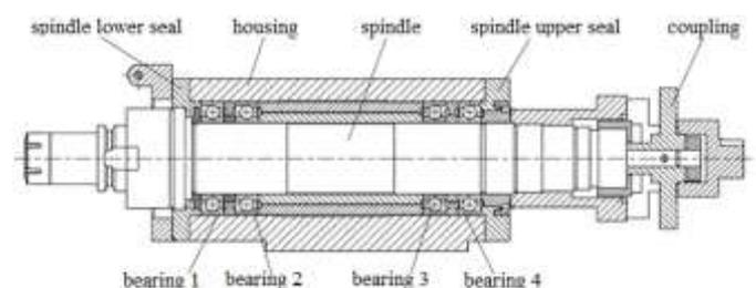
Fig. 1. Slice section of original main spindle.
