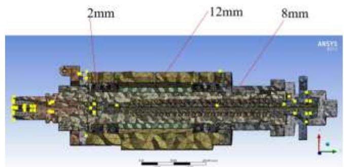
Fig. 5. The finite element model for analyzing heat transfer in the vertical spindle of a CNC milling machine.
