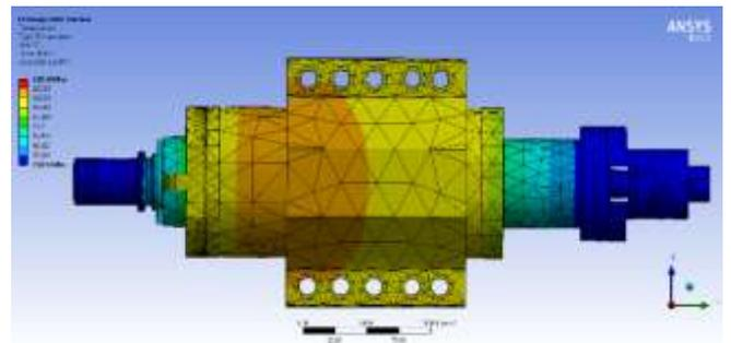
a. Thermal distribution on spindle outer case.
