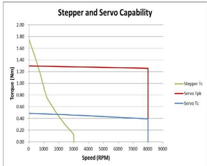
Fig. 2. Performance Curve Comparison with approximately same volume
