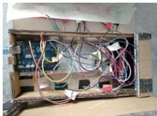
Fig. 5. Circuit connection of Arduino, Stepper motor and Servo motor
