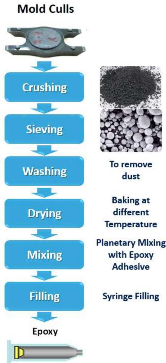
Fig. 3. Mold Cull Spacer replenishment Process for Die Attach Adhesive
