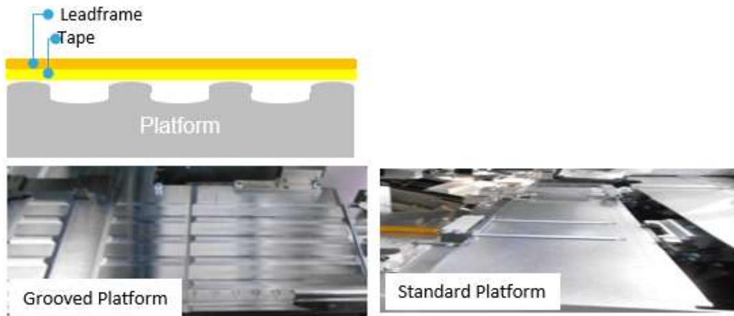
Fig. 3. Semiconductor leadframe platform augmentation.
