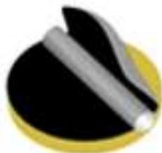
Fig. 2. Coating film lamination to wafer backside.
