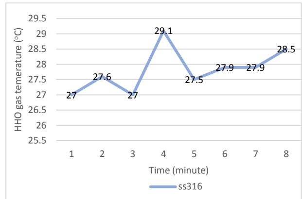
Fig. 5. Graph of HHO gas temperature with time
