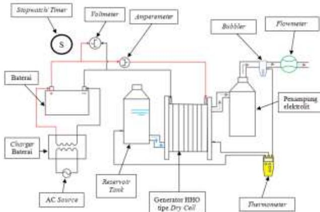
Fig. 1. HHO generator testing scheme
