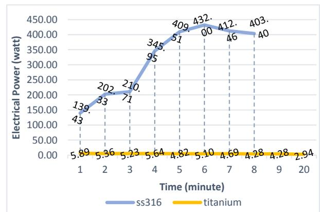
Fig. 2. Graph of power consumption with time
