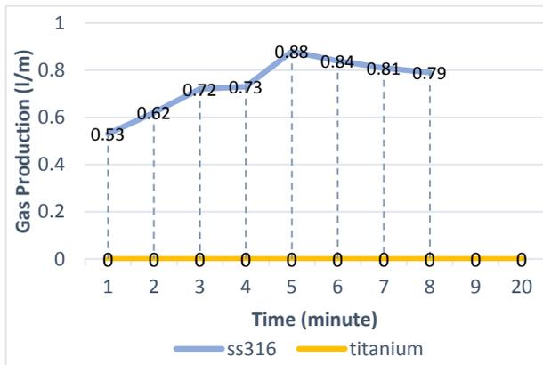
Fig. 3. Graph of HHO gas flowrate production with time
