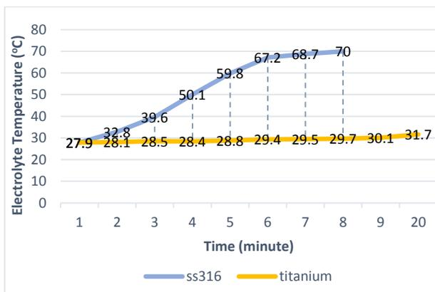
Fig. 4. Graph of electrolyte temperature with time
