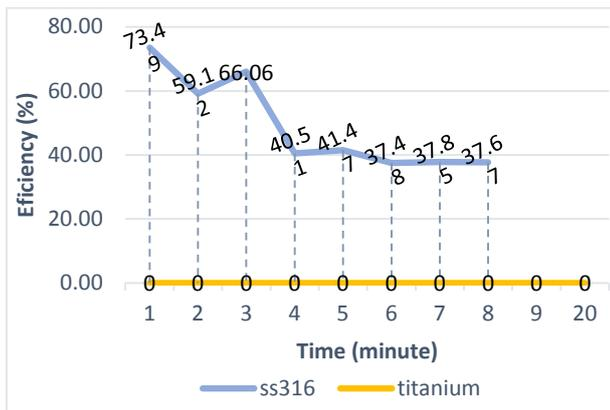
Fig. 7. HHO generator efficiency with time
