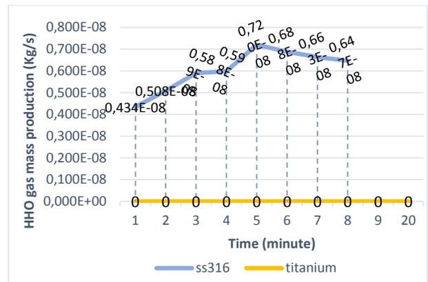
Fig. 6. Graph of HHO gas mass flowrate production with time
