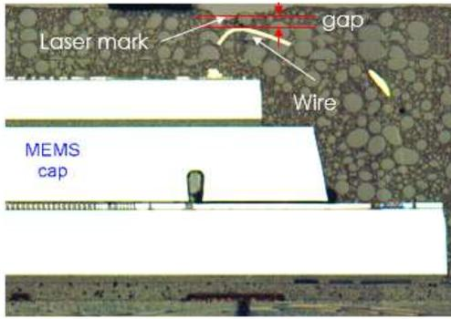
Figure 4. Cross section for gap between laser depth and wire
