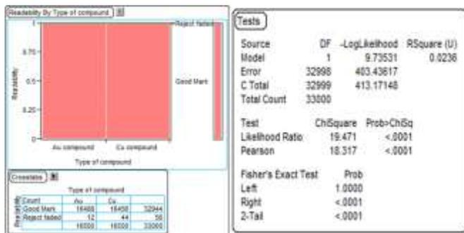
Figure 5. 2-Proportional test of mark quality between mold compound for gold wire against copper wire products
