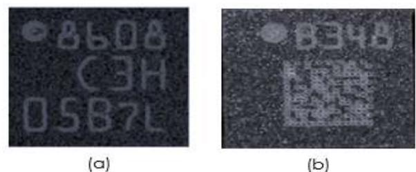
Figure 3. Laser marking on molded IC (a) Alphanumeric (b) 2D coded
