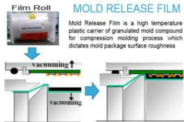
Figure 7. Mold release film in compression mold
