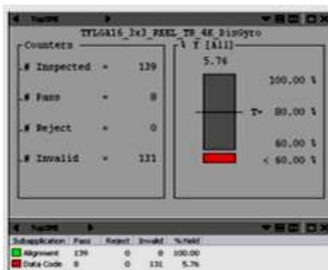
Figure 6. Mark scan failures
