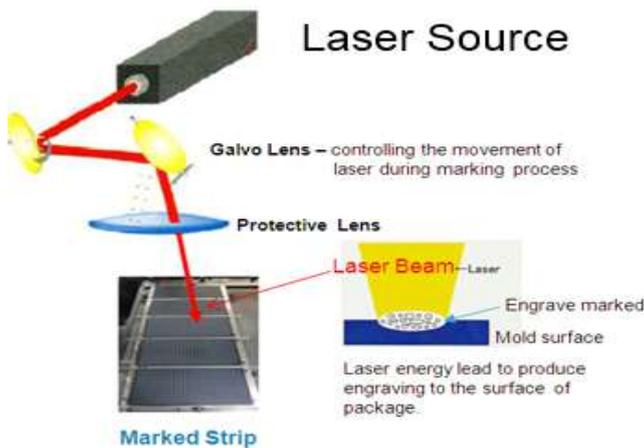
Figure 1. Laser Marking Process
