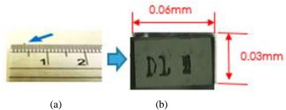
Figure 2. (a) Scalable package (b) Package/Mark Size
