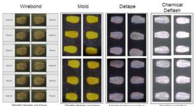
Figure 11. Lead visual after each assembly step
