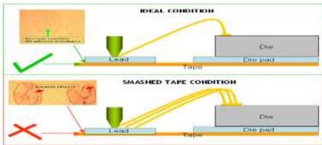
Figure 5. Tape delamination visual comparison for 1 wire on lead against 3 wires on lead
