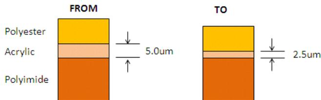
Figure 12. Illustration of the layer difference between the current and modified tape
