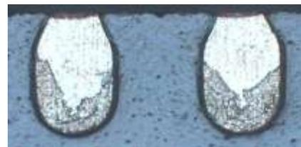
Figure 3. Actual picture of leads with tape residue and moldflash
