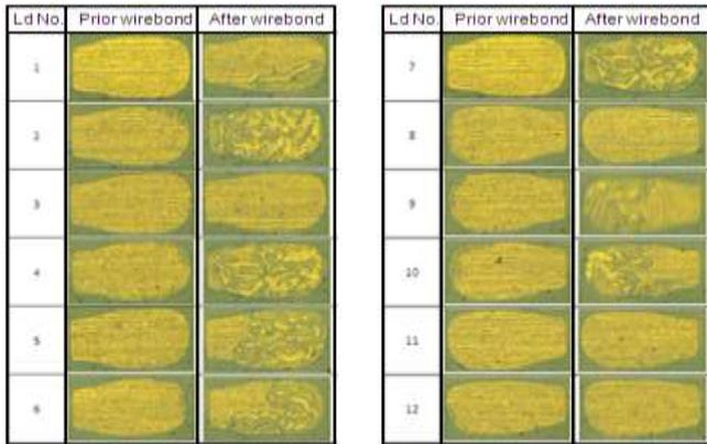
Figure 4. Tape delamination mapping before and after wirebond per lead
