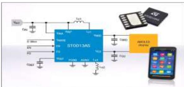
Figure 1. Schematic diagram of the STOD13AS device on a VFDFPN12 package
