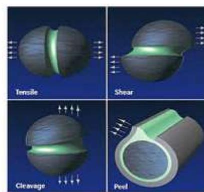
Figure 6. Different tape stress illustration
