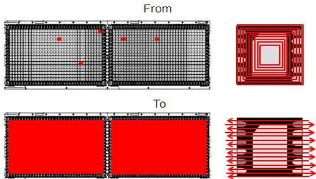
Figure 8. Laser deflash mark layout comparison
