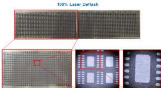
Figure 9. Actual appearance of removed moldflash via laser deflash process
