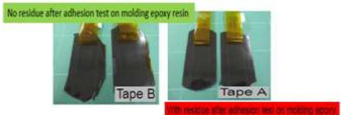
Figure 10. Laboratory test result by tape supplier
