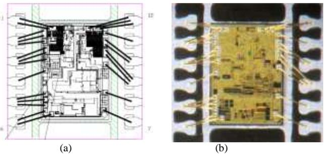
Figure 2. (a) Wirebonding layout configuration and (b) actual bonding appearance of device STOD13ASTPURSV1 on a VFDFPN12 package
