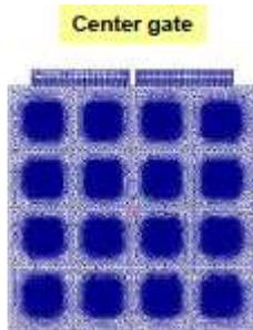
Fig. 4. Finite elements mesh generation for center gate type
