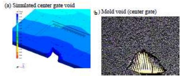
Fig. 7. The comparison of the simulated and actual mold voids
