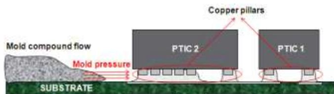
Fig. 24. Illustration of mold flow on copper pillars
