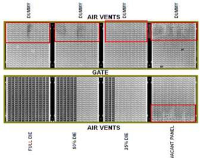
Fig. 16. SCAT response to different vacant pad quantity
