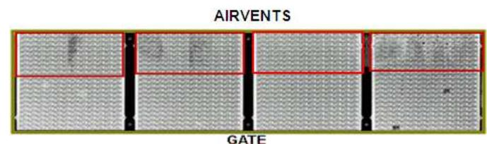
Fig. 3. Package voids localization on strip
