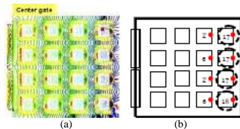
Fig. 8. (a) Mold filling time contour plotting (prediction) and (b) the actual mold void position through experiments (about 200 unit tests for each gate type)
