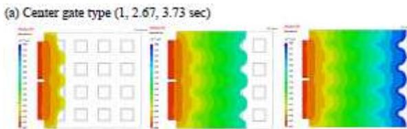
Fig. 5. Melt front advancement of evaluated gate type
