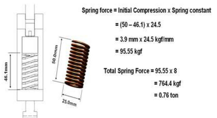
Fig. 21. Computation of spring force
