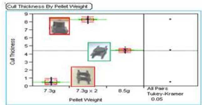
Fig. 19. Boxplot of cull thickness per pellet weight
