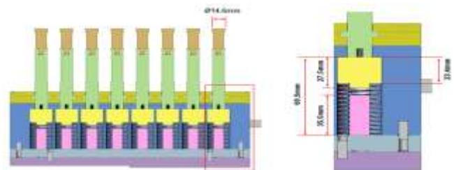
Fig. 20. Structure of transfer plunger
