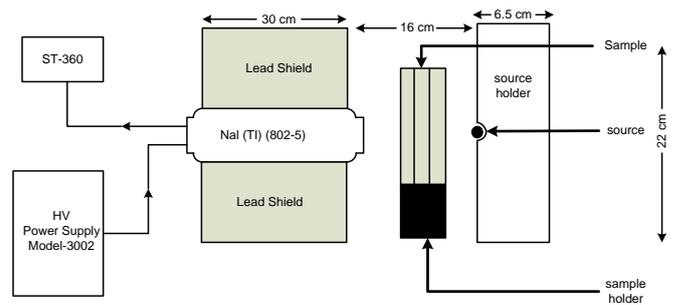
Fig. 1. Block Diagram of Experimental set up
