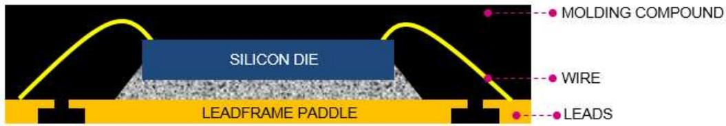
Fig. 2 Cross-sectional illustration of a standard leadframe-based device.
