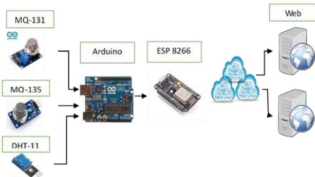
Figure 1. Air Monitoring Diagram System
