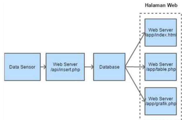
Figure 2. Block Diagram of Monitoring System
