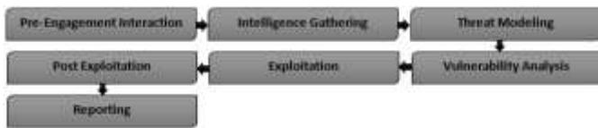
Fig. 1. Stages of Penetration Testing
