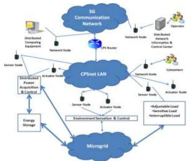
Fig. 2: Cloud computing model for smart grid
