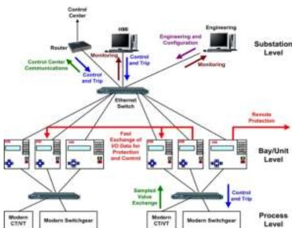
Fig. 4: Configuration of substation automation system
