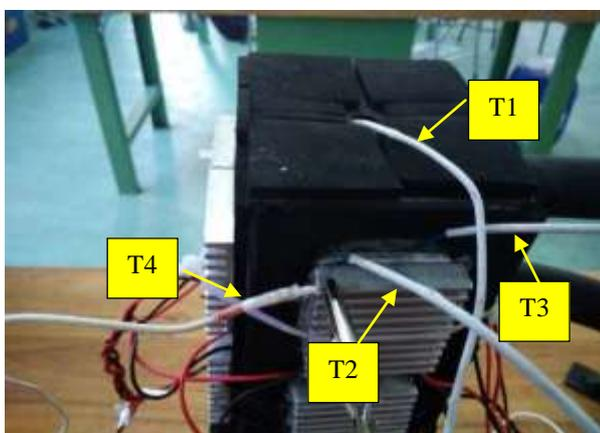
Figure 6. Schematic of a thermocouple mounting circuit for temperature measurement
