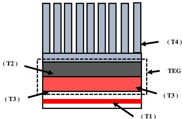
Figure 5. A series of thermocouple installations for temperature measurement
