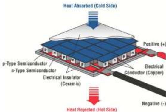
Figure 3. Structure of Thermoelectric Generator Elements
