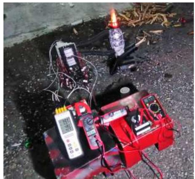
Figure 8. TEG SP1848 type thermoelectric testing process
