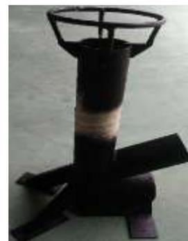
Figure 1. Rocket Stove with a ratio of upright and horizontal sides is 3: 1
