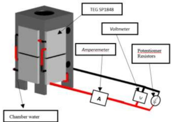
Figure 7. Schematic of a power data collection circuit with resistor potentiometer resistance in TEG
