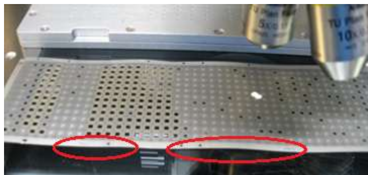
Fig. 3. Leadframe strip warpage after wirebond process.
