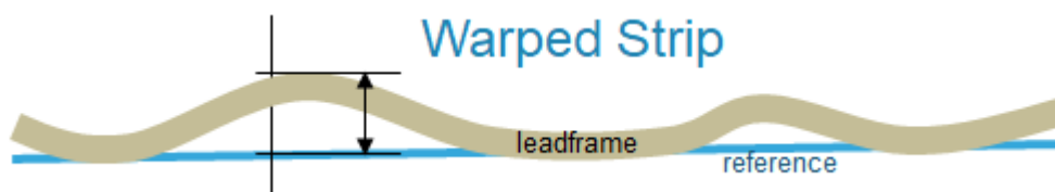
Fig. 1. Strip warpage representation.
