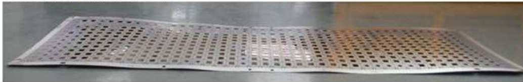
Strip warpage prior Mold process
