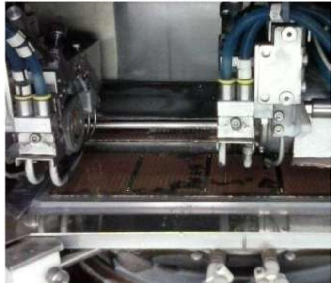
Fig. 2. Mechanical package singulation
