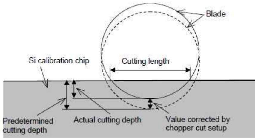
Fig. 3. Chopper Cut Set-up [6]
